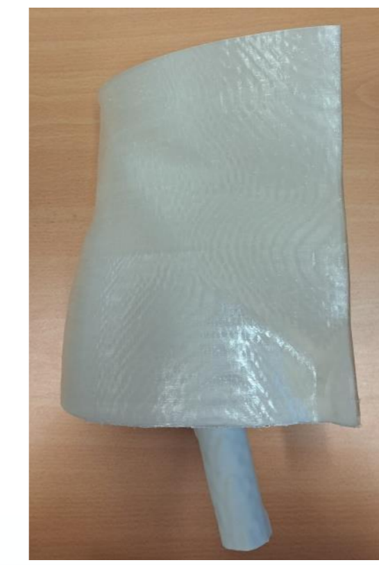
Figure 8: 3D printed femur within 3D printed side module
