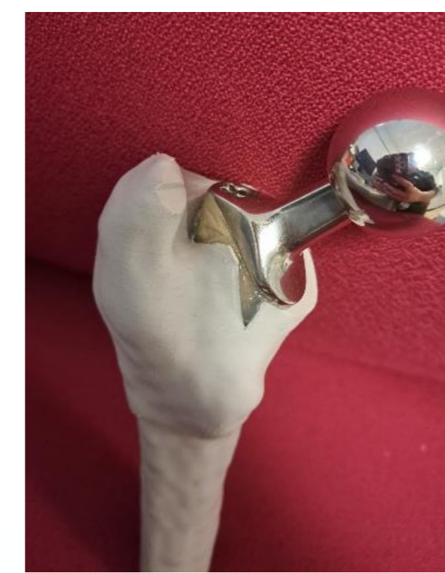
Figure 7: 3D printed femur with metal hip implant:
